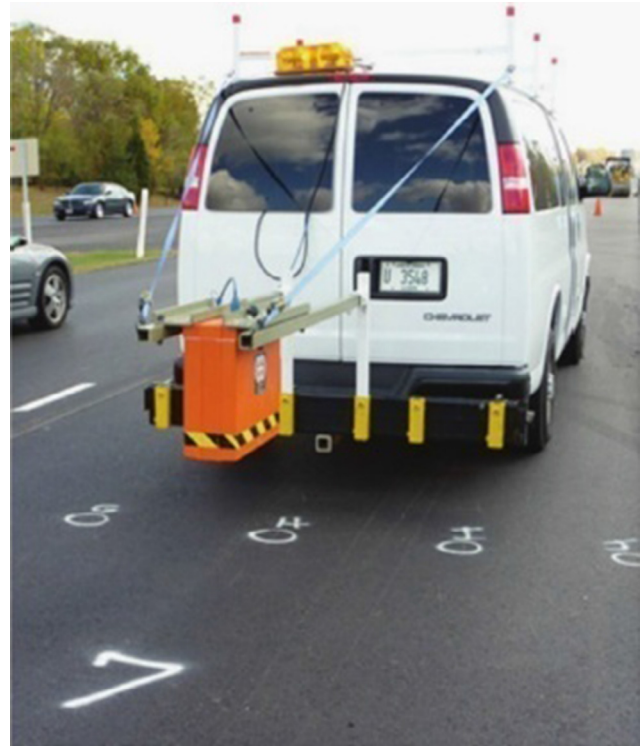
Fig. 1. GPR inspection of an asphalt pavement using an air-coupled TEM horn antenna.
